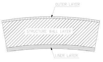
GRP pipe is a composite laminate consisting of mainly three layers. The first layer is a corrosion resistant liner called the inner liner, the second layer is the structure layer, and the external layer is a resin rich layer.
